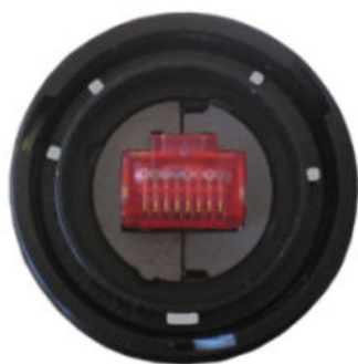
Fig. 2-8: RJ-45 connector in housing as required by Code C
