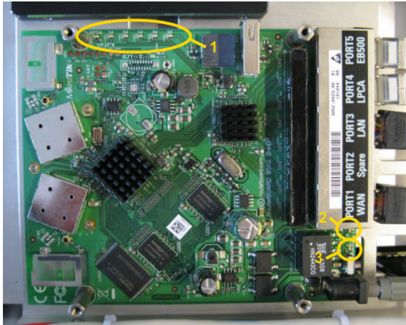
Fig. 4-25: LEDs on the router board
