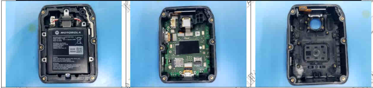
VBWAZS0183 (Disassemble and inspect, no dust enters the inside of the sample)
