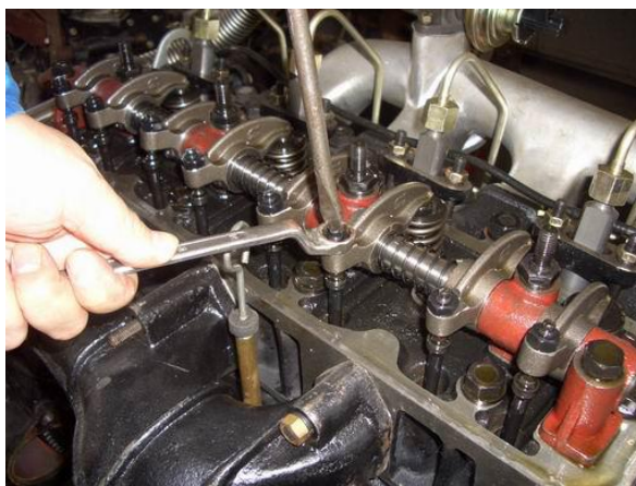
Figure 2-7 Adjustment of valve clearance
