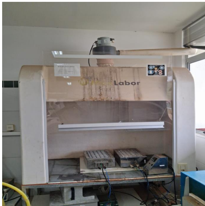
Figura 59 – Vista frontal bloco digestor SL 25/40.
