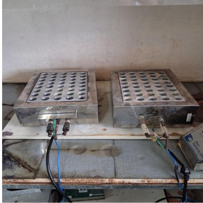
Figura 60 – Vista interna bloco digestor SL 25/40.
