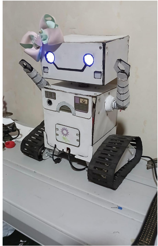
Fig. 1: Physical prototype of the social robot constructed with cardboard and PVC.
