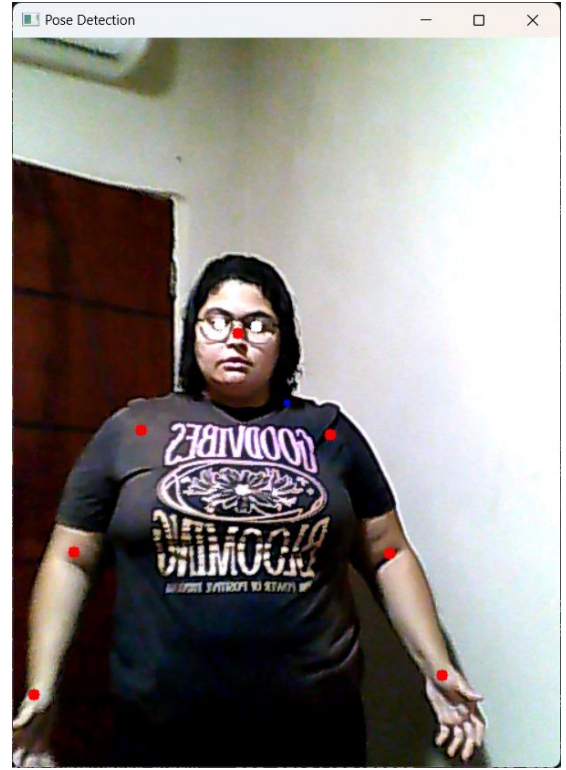
Fig. 2: Visualization of pose and face landmarks used for gesture and distance estimation. Red points represent pose landmarks, while white points denote irises, and the blue dot indicates the image center.
