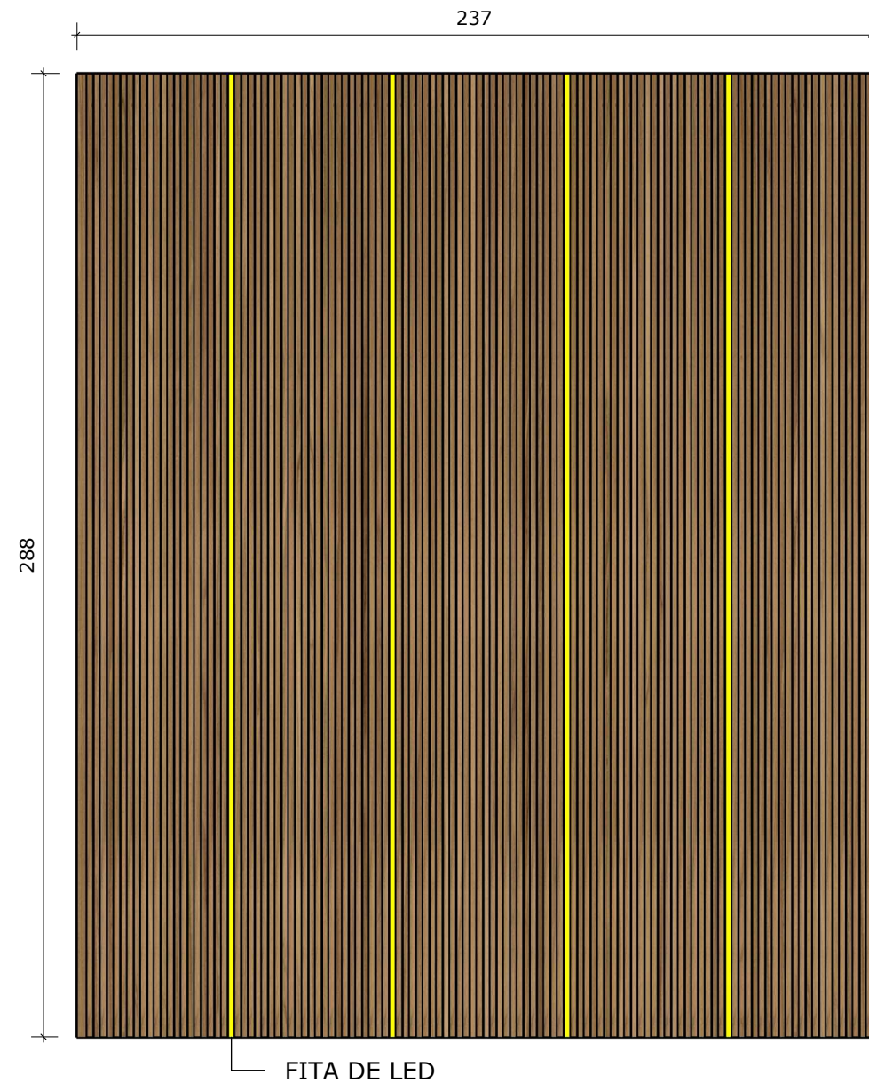
VISTA FRONTAL- PAINEL RIPADO ESCALA 1:20
